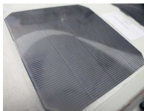
Figure 1: An integrated sintered substrate, the conductive zones (in clear) are separated by insulating areas (in dark)
